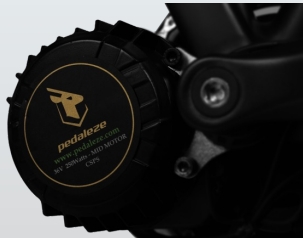
DMT-250-MAC powerful Mid drive with 90Nm of torque for a smooth and effortless travel
